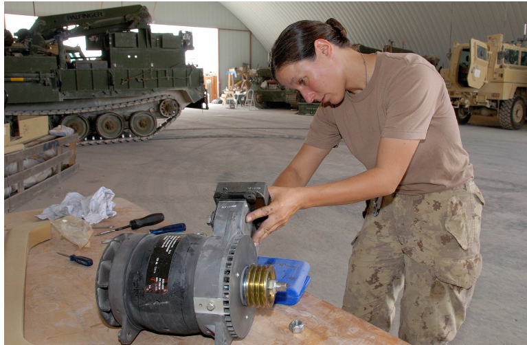
Vehicle technician Corporal Heather Skaling of the National Support Element repairs the alternator in a LAV III light armoured vehicle at Kandahar Airfield.
